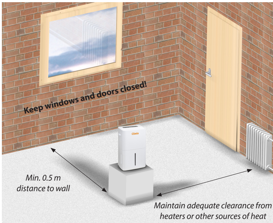
Fig. 2 Schematic depiction of how to set up the air dehumidifier
