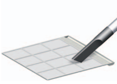
Fig. 9 Cleaning with a vacuum cleaner
